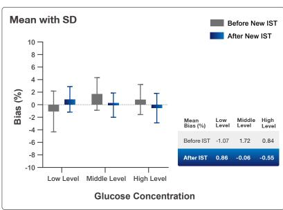
**Precision:** for each glucose interval, the test results obtained from Diamond BGMS were calculated to determine its Mean, Standard Deviation (SD), and Coefficient of Variation (CV%)
