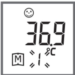
When the memory is full, the oldest result is deleted as the new one added. When the last record is displayed in the LCD, press On / Memory button again to return the first record.
