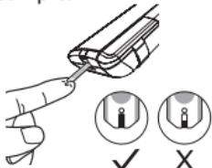
Move your finger to meet the absorbent hole of the test strip and the drop will be automatically be drawn onto the test strip. Remove your finger until the confirmation window is filled. The meter begins to count down. Do not remove your finger until you hear a beep sound.
