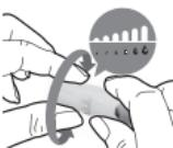
6. Pull the cocking control out until the orange bar appears on the release button window.
