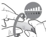
6. Pull the cocking control out until the orange bar appears on the release button window.
