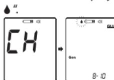
2. Press **▲** to adjust the measuring mode, and press **MAIN** button to confirm it.
